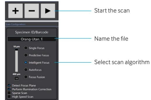
**Predictive Focus:** The computer automatically sets focus points, calculates a focal plane and scans the area by taking one image per x-y position.
