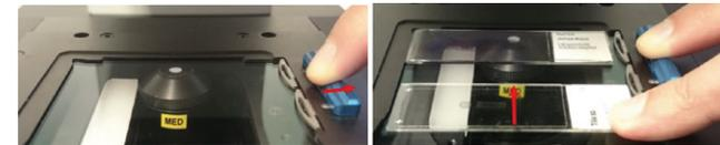
Repeat this step to insert a second slide. When all slides are mounted, release the handle. The slide mount closes automatically.
